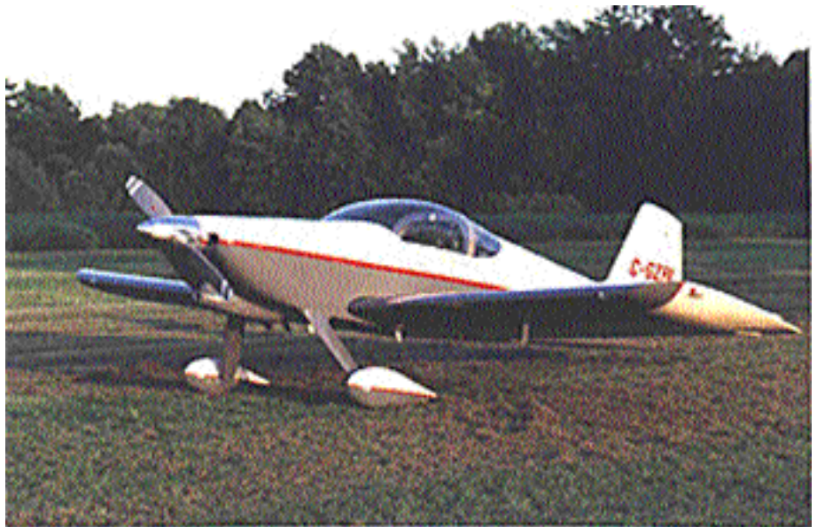
Terry completed C-GZRV in 1998, and won an Outstanding Workmanship award at Oshkosh. The airplane has a fuel-injected, 180 hp O-360 and a CS prop.
