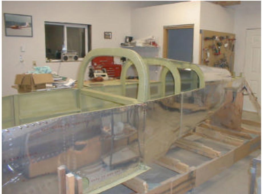
fuselage close to the floor for work height convenience. The jig allowed me to level the fuselage and cross brace at the tail end from the top of the rear fin attachment area (Bulkhead F612) down to each side of the jig. To hold the front end I placed the wood wing spar simulators in place, bolted
